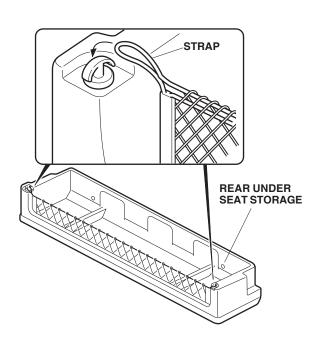
6. Position the rear under seat storage on the carpet, and align the holes in the rear under seat storage with the holes in the brackets. Secure the seat storage with the two knob bolts.
